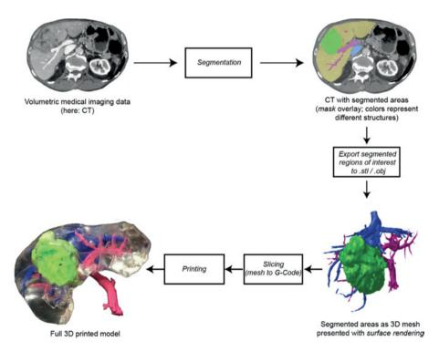
Fig. 5.1: Workflow of 3D printing: all phases from image acquisition to printed model. Case of 3D printing liver models for preoperative planning, done routinely at Jagiellonian University (Kraków, Poland).
