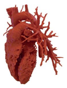
Fig. 5.4: Fused deposition modeling approach allows labs to create personalized models of congenital heart diseases with approximately 24-h turnaround time from image acquisition. This fabrication technique was satisfactory here, as models are used only for visualization and not for simulation. The model in this picture was delivered to cardiologists from University Children's Hospital of Kraków.
